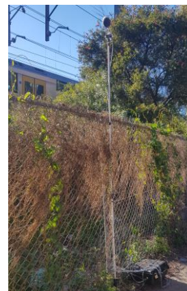
Figure4: Location of vibration Ground Vibration Accelerometer
