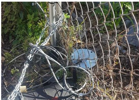
Figure4: Location of vibration Ground Vibration Accelerometer
